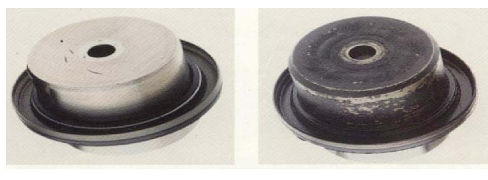
Thermally stable gear lubricants resist oxidation and decomposition, preventing deposits on seals which can lead to seal failure and lubricant loss.
